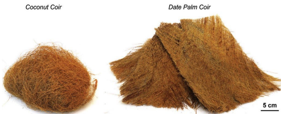
Visual Comparison of Coconut Coir Fiber (left) after extraction and processing, and Date Palm Fiber (right) before fiber processing (separation).
