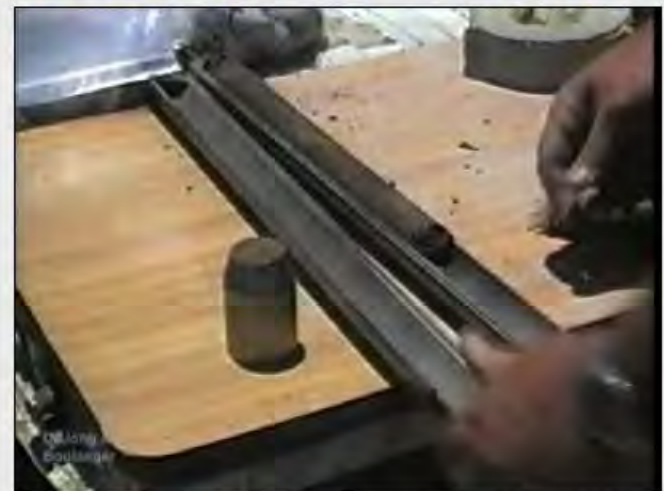
Split Spoon Sampler in Open Condition Showing Recovered Sample
